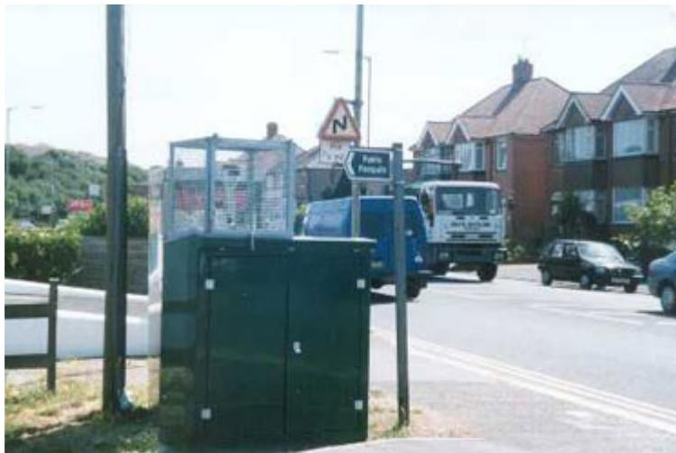
The Council previously operated a separate roadside site; Hastings - Freshfields, which was adjacent to Bulverhythe sports pavilion. Monitoring of NO<sub>2</sub> and PM<sub>10</sub> at this site started in 2008 and ended in 2011. The sample inlet was approximately 2m from the kerb. (See <http://www.sussex-air.net/AQNearMe/Monitoring/SiteDetails.aspx?SiteCode=HT2&SiteName=Hastings%20-%20Fresh%20Fields>)
