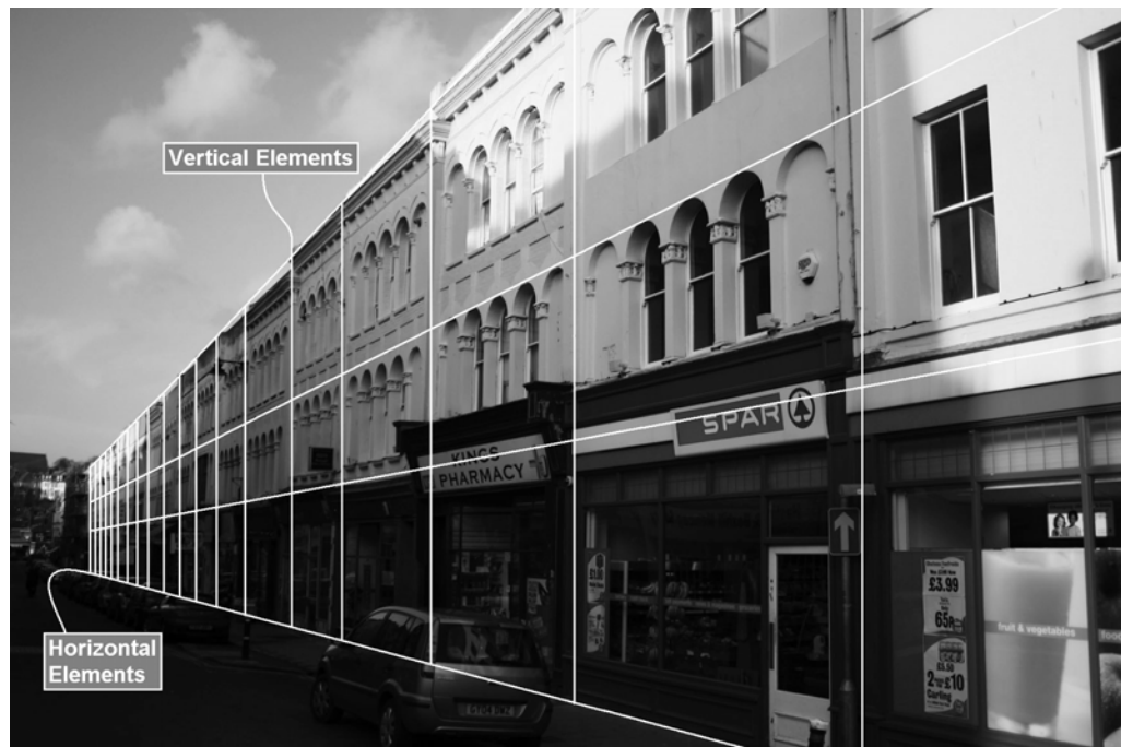
Diagram showing the vertical and horizontal elements of a terrace of buildings
